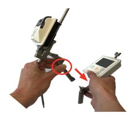
Press button on probe arm and place onto jig [Ensure rear of jig is supported while attaching]
