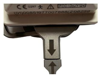
Align arrows on sensor and impactor adapter
