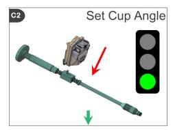
Attach sensor to impactor
